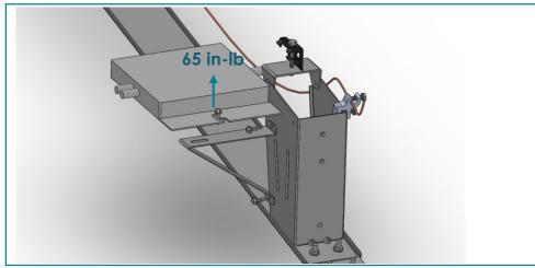
To attach an accessory to the AMP, use a 1/4-20 Stainless Steel Bolt with a Stainless Steel Star Lock Washer and a Stainless Steel Serrated Hex Flange Nut.
