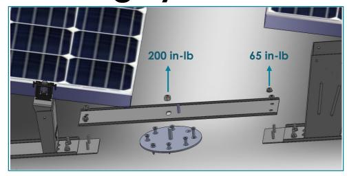
The Seismic Attachment Plate (SAP) is connected to the system through the center hole of the Connect Belt and Connect Belt Extension. Not every Connect Belt will need an SAP. Consult a qualified structural engineer to determine quantity and placement of SAPs. Tighten 3/8 Serrated Hex Flange Nut to 200 in-lb.
