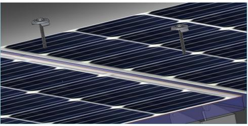
Insert 1/4-20 x 2" Stainless Steel Hex Cap Bolts through one lock and one flat washer and then through the Stainless Steel Grounding Mid Clamp Cap.
