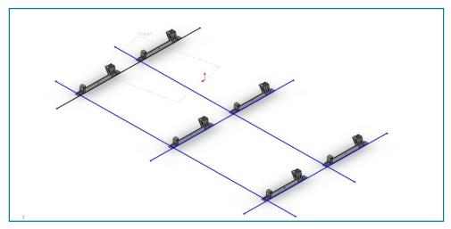
Align pre-assembled High, Low Bracket and solar belt combination with pre-drawn chalk lines.
