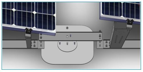
Insert **Bolts** into the threaded PEM Nuts in the top of each U-Anchor as shown and tighten to **65 in-lb.**
