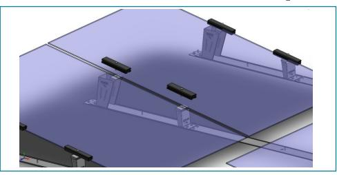
Insert 1/4-20 x 2" Stainless Steel Hex Cap Bolts through one lock and one flat washer and then through the Stainless Steel Grounding Mid Clamp Cap.
