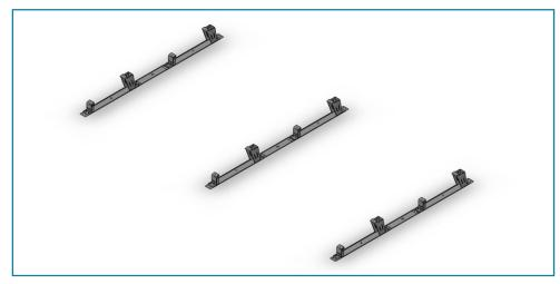
Add Connect Belts between each row over the top of the brackets on the PEM Studs. Add a 1/4-20 Stainless Steel Serrated Hex Flange Nut to each PEM Stud and tighten to 65 in-lb.
