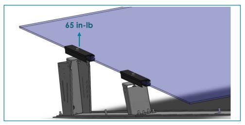
Panel should be centered over brackets with equal overhang on each side.
