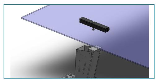
Place PV Module on brackets and line Grounding End Clamps up to span both brackets...
