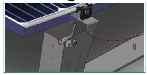
Ground lugs should be placed before PV Modules are installed. Apply lug to the edge of a high or low bracket as shown above.
