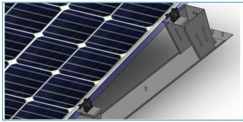
Place PV Module on brackets and line Grounding End Clamps up to span both brackets..
