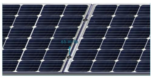
Place PV Module on brackets and line Grounding End Plate up to span both brackets.
