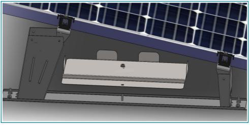
Place the Side Ballast Pan over the Solar belt.
