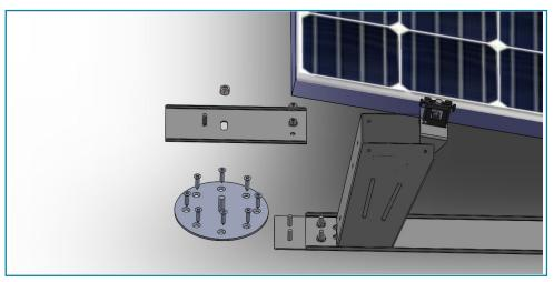
Replace the connect belt /connect extension on the system and secure the 1/4-20 Serrated Hex Flange Nuts to 65 in-lb.
