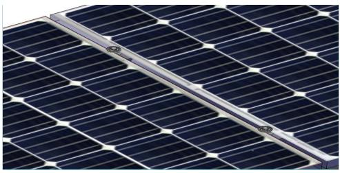
Insert Bolts into the threaded PEM Nuts in the top of each bracket as shown and tighten to **65 in-lb.**
