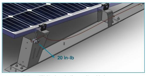
As a general rule, one SGB-5 Lug is required for every **56 modules** in array. Bolts should be torqued to **20 in-lb**.
