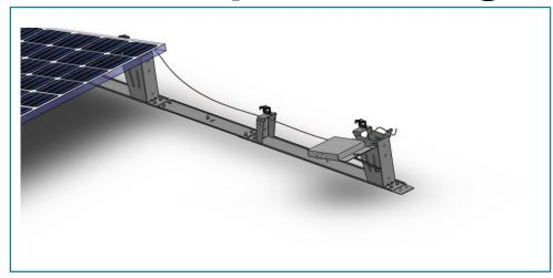
The Accessory Mounting Plate (AMP) should be attached to either side of the High Bracket using up to  $4 \times \#10$  Stainless Steel Self Tapping Sheet Metal Screws.
