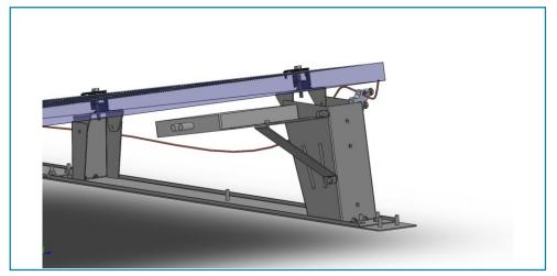
Attach the accessory using the slot on the top of the AMP. tighten bolt to  ${\bf 65}$  in-lb.
