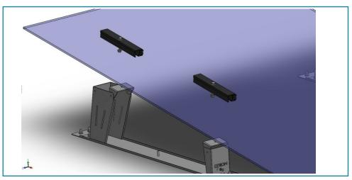
Insert 1/4-20 x 2" Stainless Steel Hex Cap Bolts with stainless steel flat and lock washers into the two holes in the Grounding End Ground.
