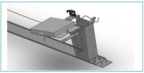
When choosing a position on the bracket, make sure that placement of ballast blocks or panels wont interfere with the attachment or the accessories being mounted to the attachment.
