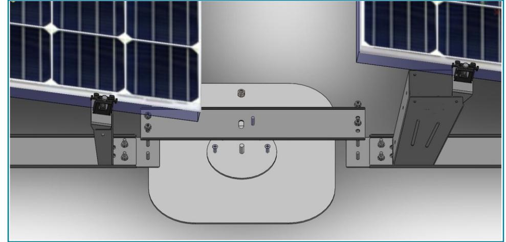
Insert **Bolts** into the threaded PEM Nuts in the top of each U-Anchor as shown and tighten to **65 in-lb**.
