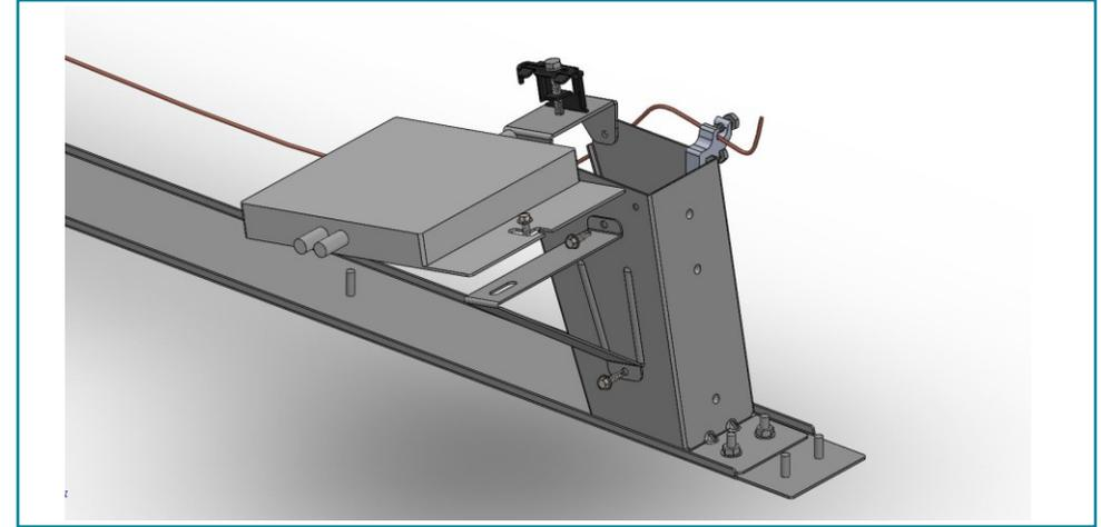
When choosing a position on the bracket, make sure that placement of ballast blocks or panels won't interfere with the attachment or the accessories being mounted to the attachment.
