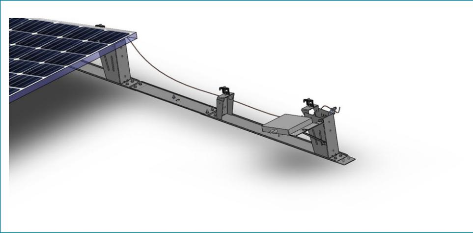
The Accessory Mounting Plate (AMP) should be attached to either side of the High Bracket using up to 4 x #10 Stainless Steel Self Tapping Sheet Metal Screws.
