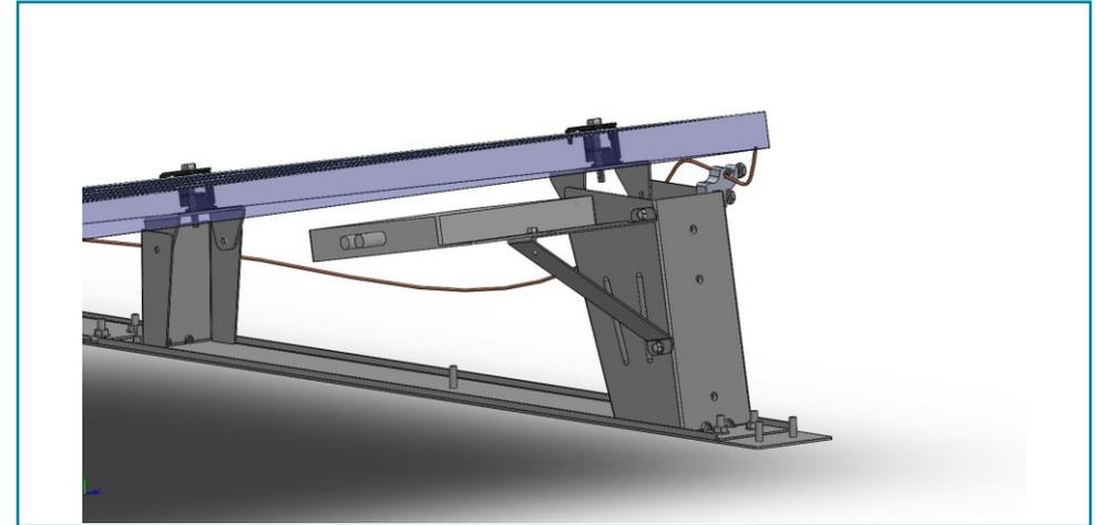
Attach the accessory using the slot on the top of the AMP. tighten bolt to **65 in-lb**.
