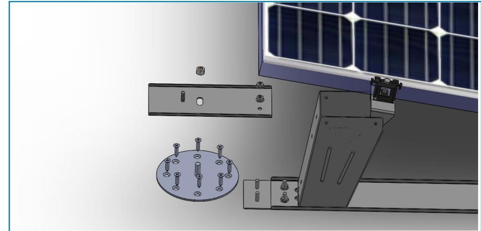
Replace the connect belt /connect extension on the system and secure the **1/4-20 Serrated Hex Flange Nuts** to **65 in-lb**.
