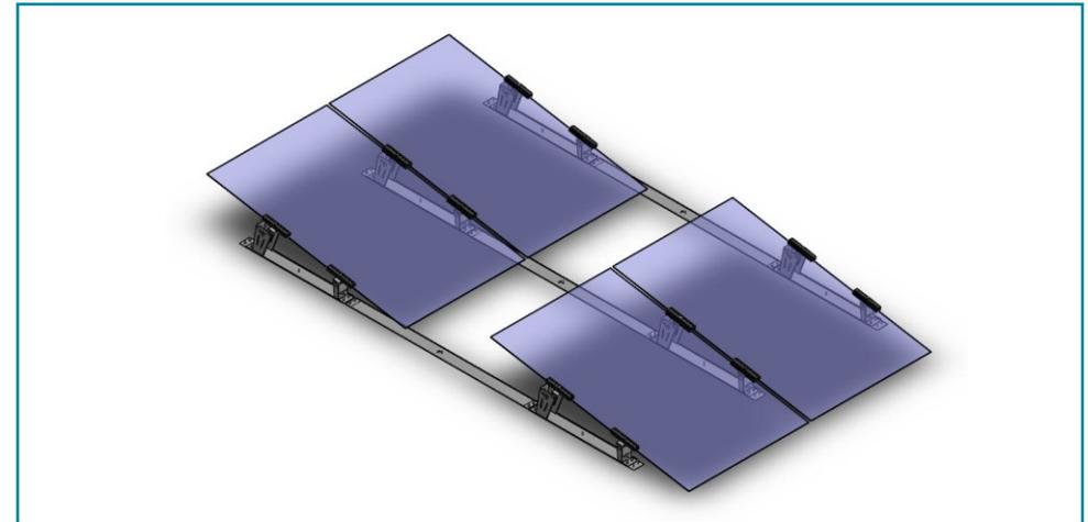
Place PV Module on brackets and line Grounding End Plate up to span both brackets.
