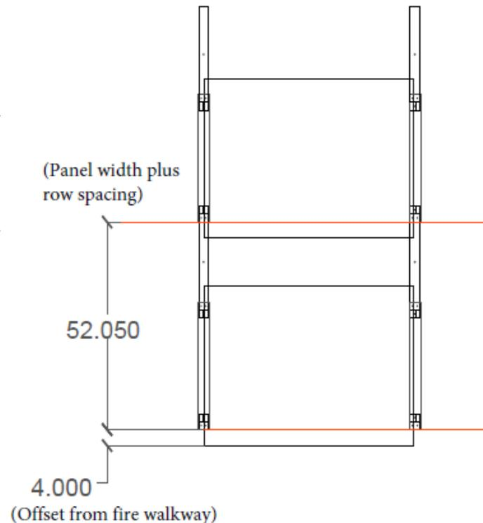
Horizontal chalk lines will mark placement of the short edge of the ballast pan (or Solar Belt).
