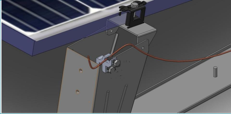
Ground lugs should be placed before PV Modules are installed. Apply lug to the edge of a high or low bracket as shown above.
