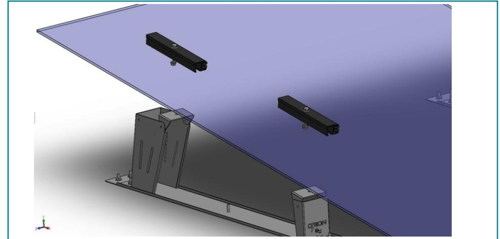
Insert **1/4-20 x 2" Stainless Steel Hex Cap Bolts** with stainless steel flat and lock washers into the two holes in the Grounding End Ground.
