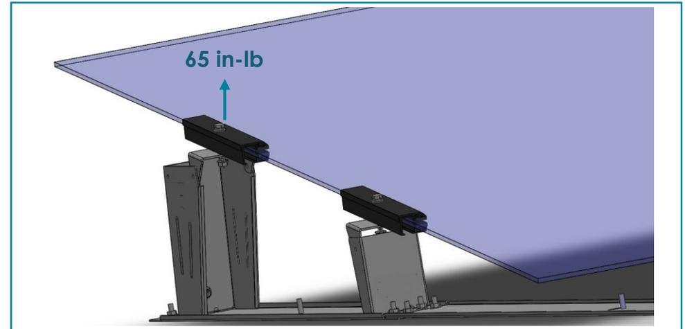
Panel should be centered over brackets with equal overhang on each side.
