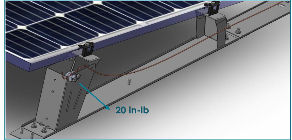
As a general rule, one SGB-5 Lug is required for every **56 modules** in array. Bolts should be torqued to **20 in-lb**.
