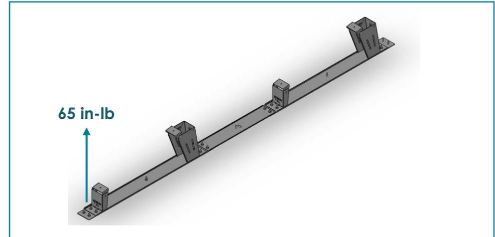
Seismic attachment plates, U-Anchors or Flash Belts have been predetermined, attach to connect belts before installing between rows. See Page 9 "Securing System" of this manual.
