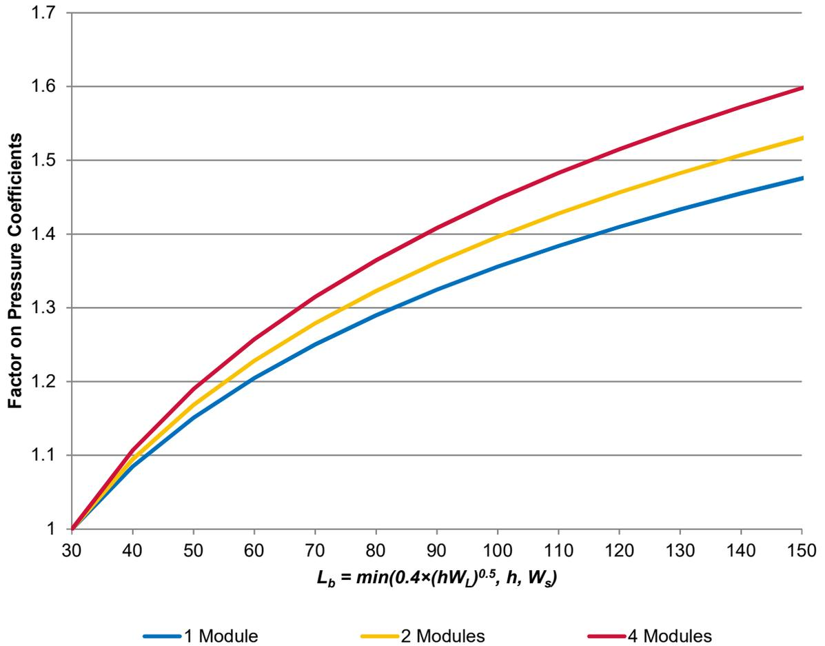
This curve is based on the curves presented in Figure 29.9-1 of SEAOC PV-2.  $h$  is the height of the building (in feet),  $W_L$  and  $W_s$  are the longest and shortest lengths of the building, respectively, (in feet).
