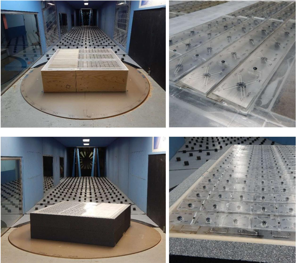
Figure 1 - Representative Wind Tunnel Models
