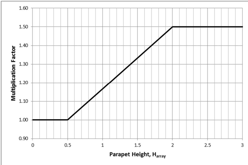
Figure 2 - Parapet Height Factor Curve
