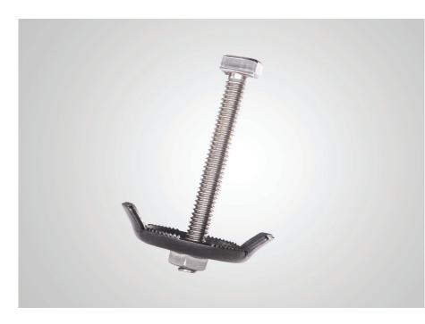
Preassebled midclamp used to clamp onto solar panels inside solar array. Made to clamp modules between 30 - 50 mm. XX can be 3035,3546 or 4550
